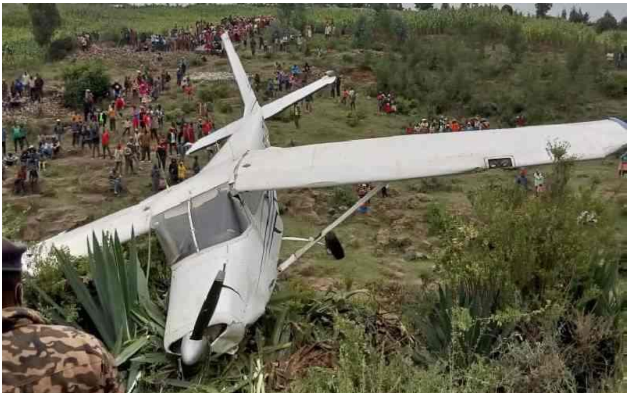
Figure 3: Photograph showing the damage of the accident aircraft at the accident site.
