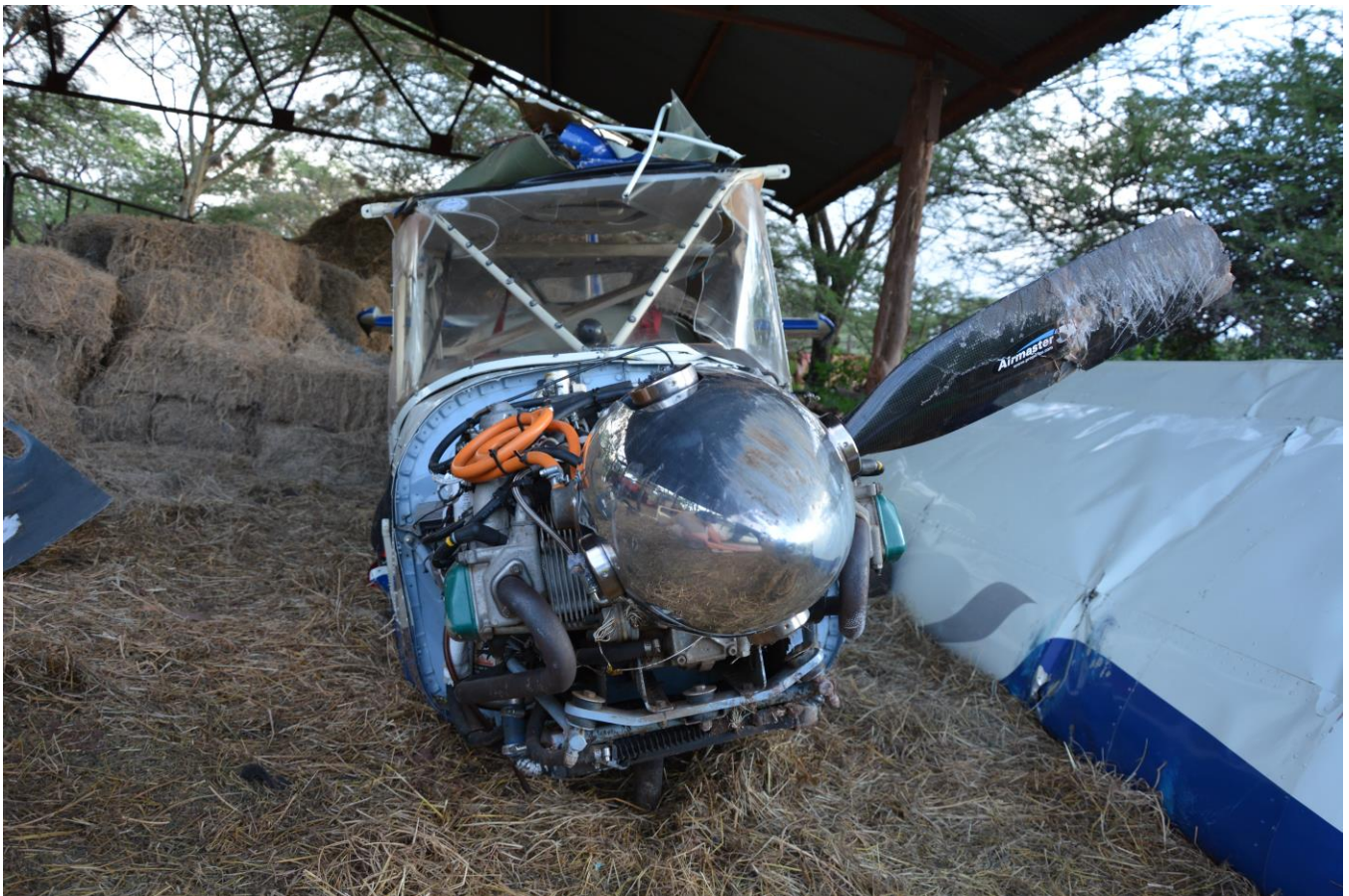
FIGURE No. 4 – A photo depicting extent of damage to the propeller, engine, cockpit area, wing and fuselage roof
