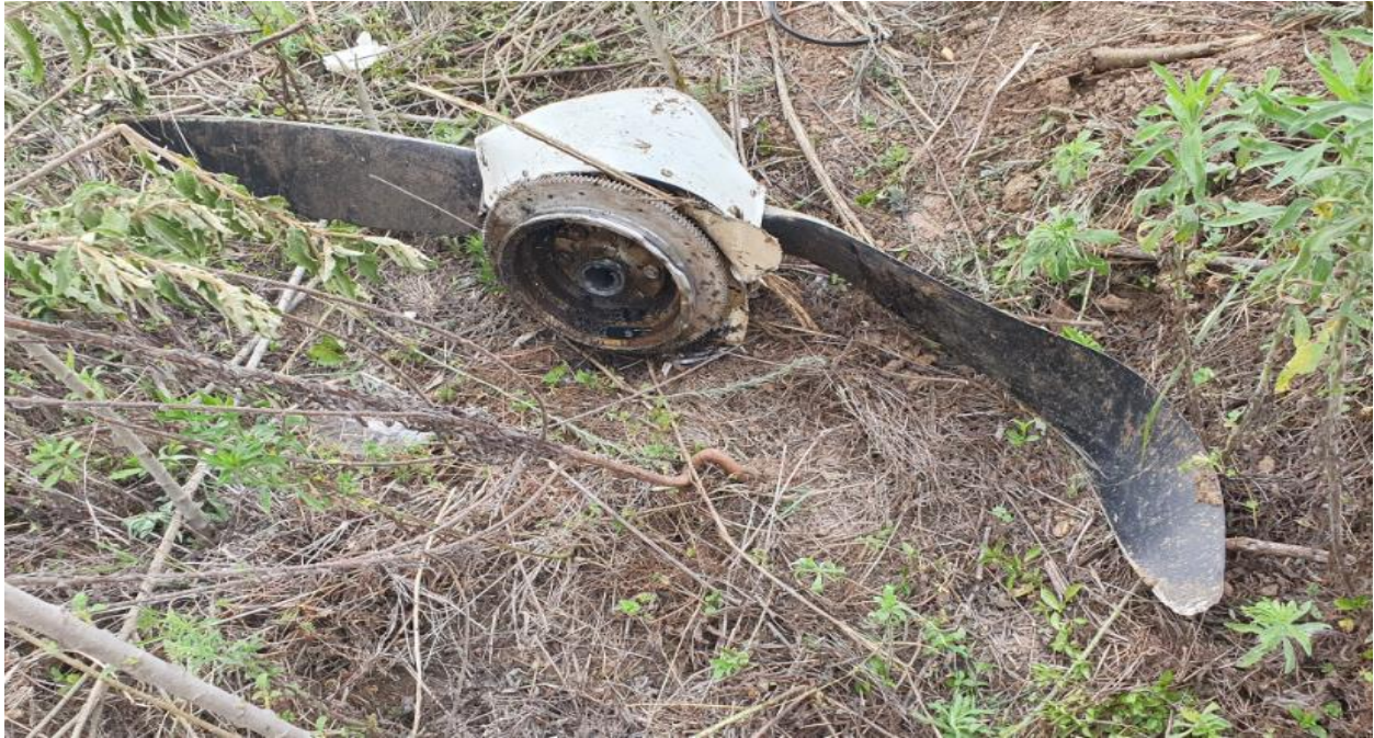
Figure 9: Damaged propeller assembly
