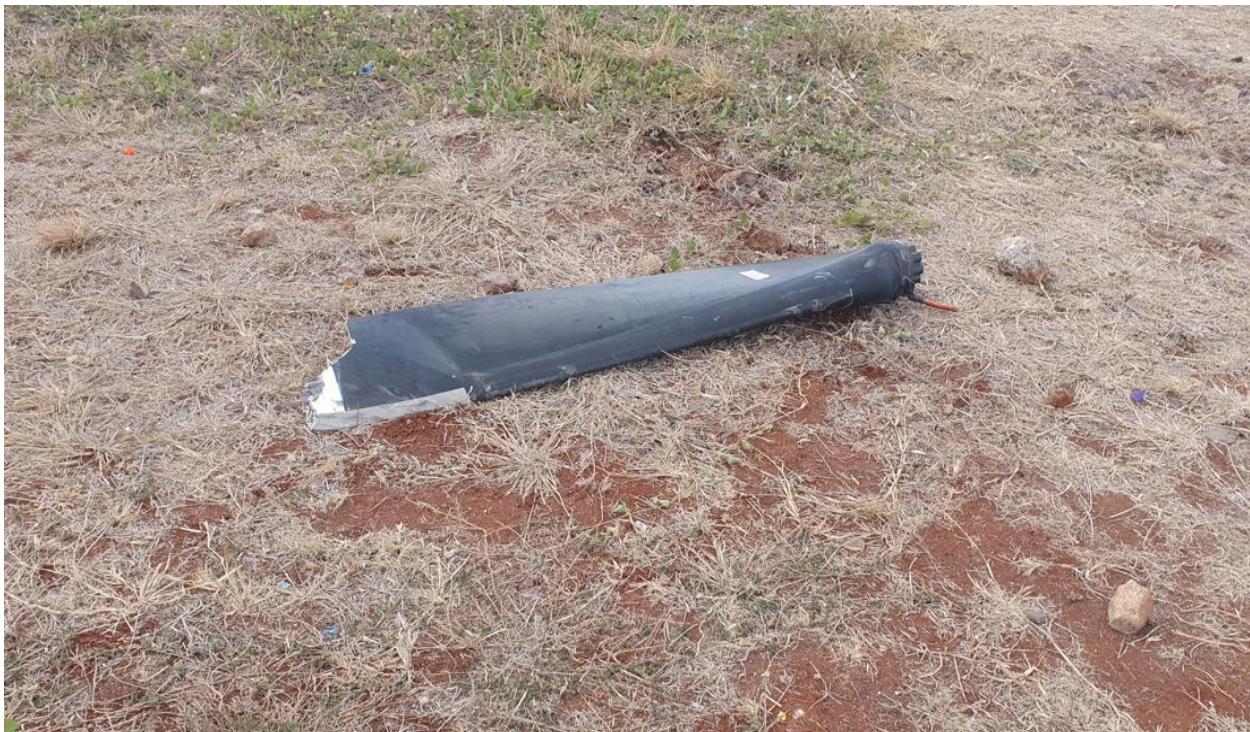
Figure 9: One of the propeller blades that separated from the aircraft
