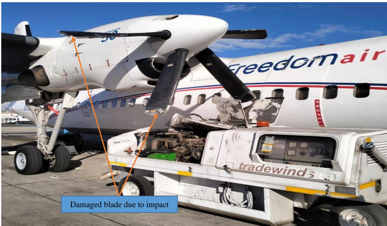
Figure 5: Damage on the R/H propeller blades
