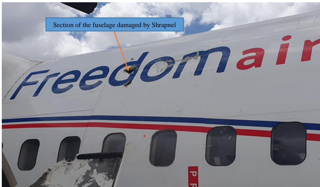
Figure 7: Fuselage penetrated by the Shrapnel.
