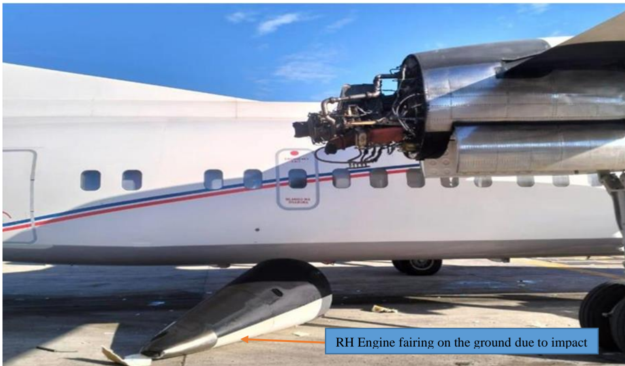
Figure 6: The RH side AFT section
