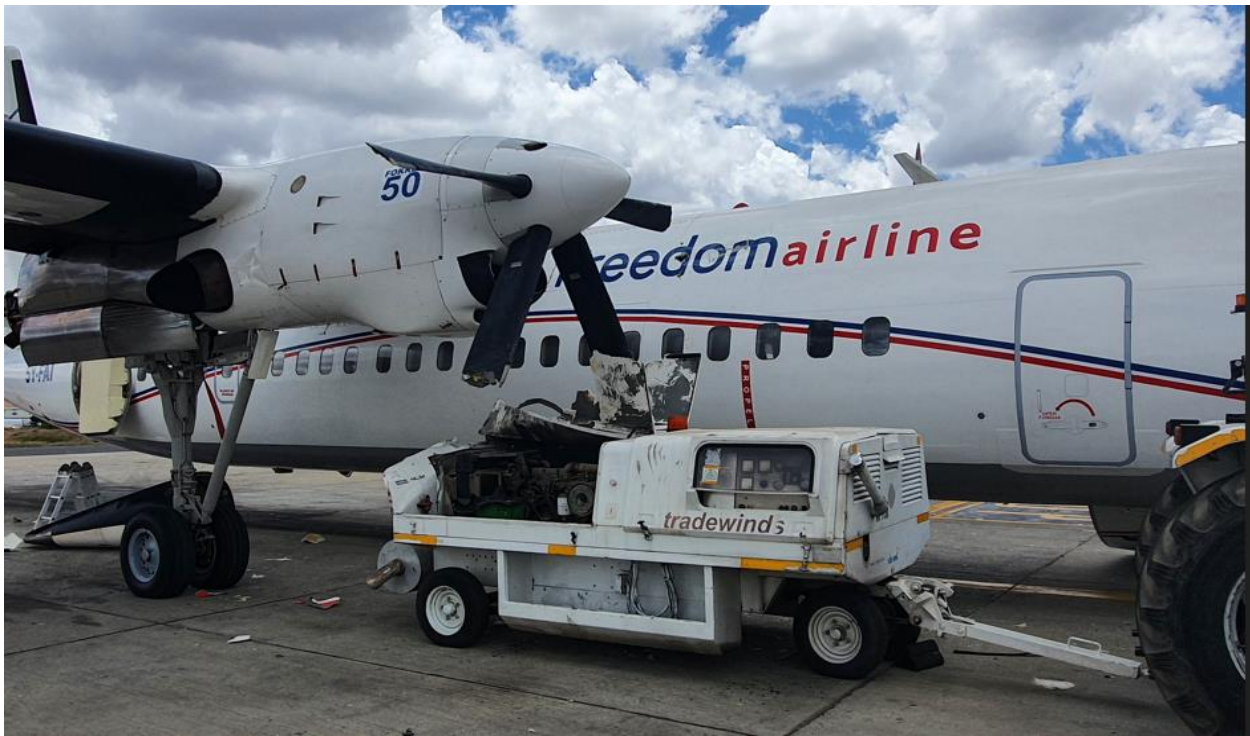
Figure 8: Damaged propeller blades and the GPU
