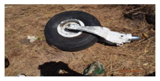
Figure 7: Photograph showing the aircraft nose-wheel that separated after impact
