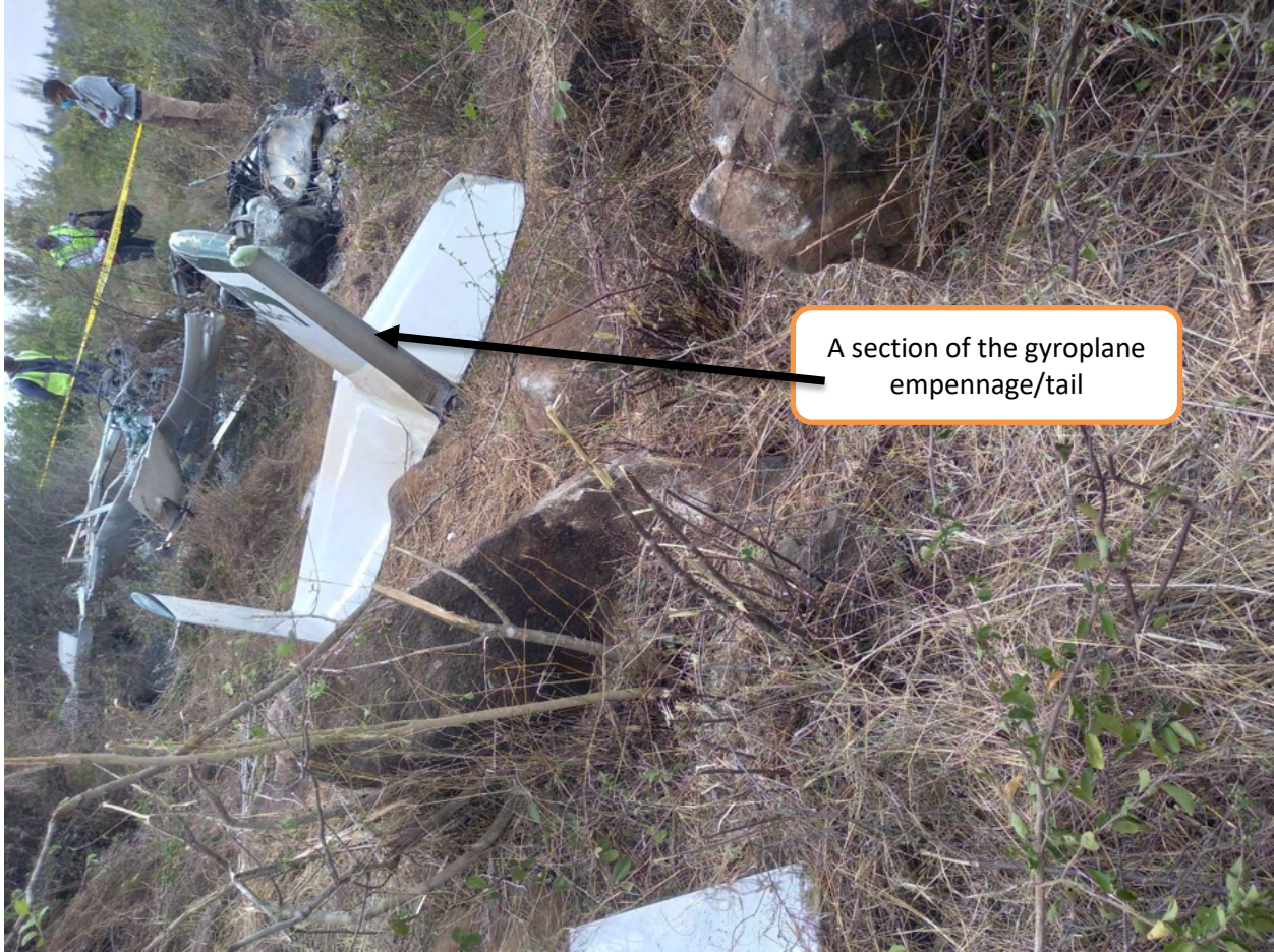
Figure 4: Photograph showing the Gyroplane empennage
