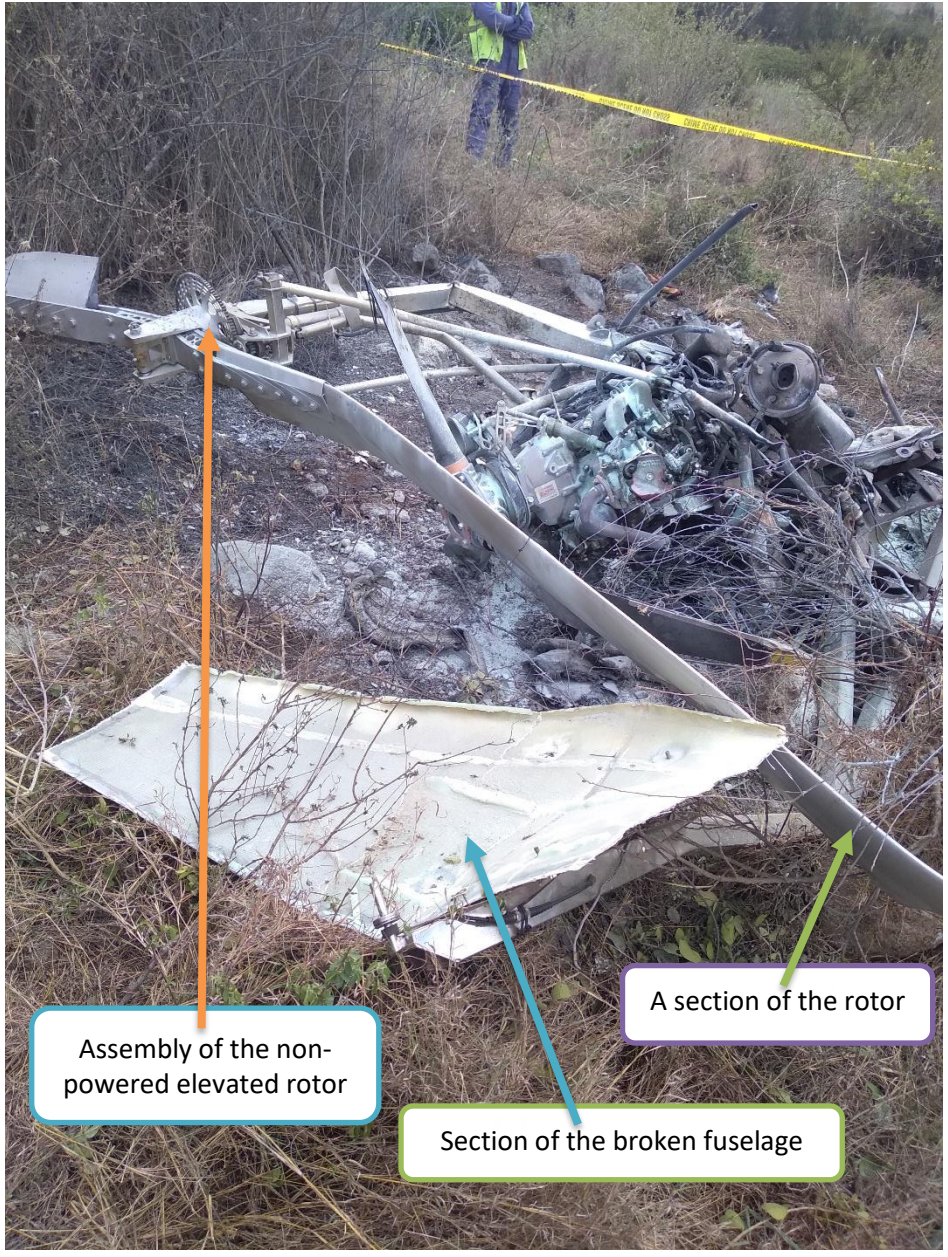
Figure 5: Photograph showing the non-powered rotor of the Gyroplane
