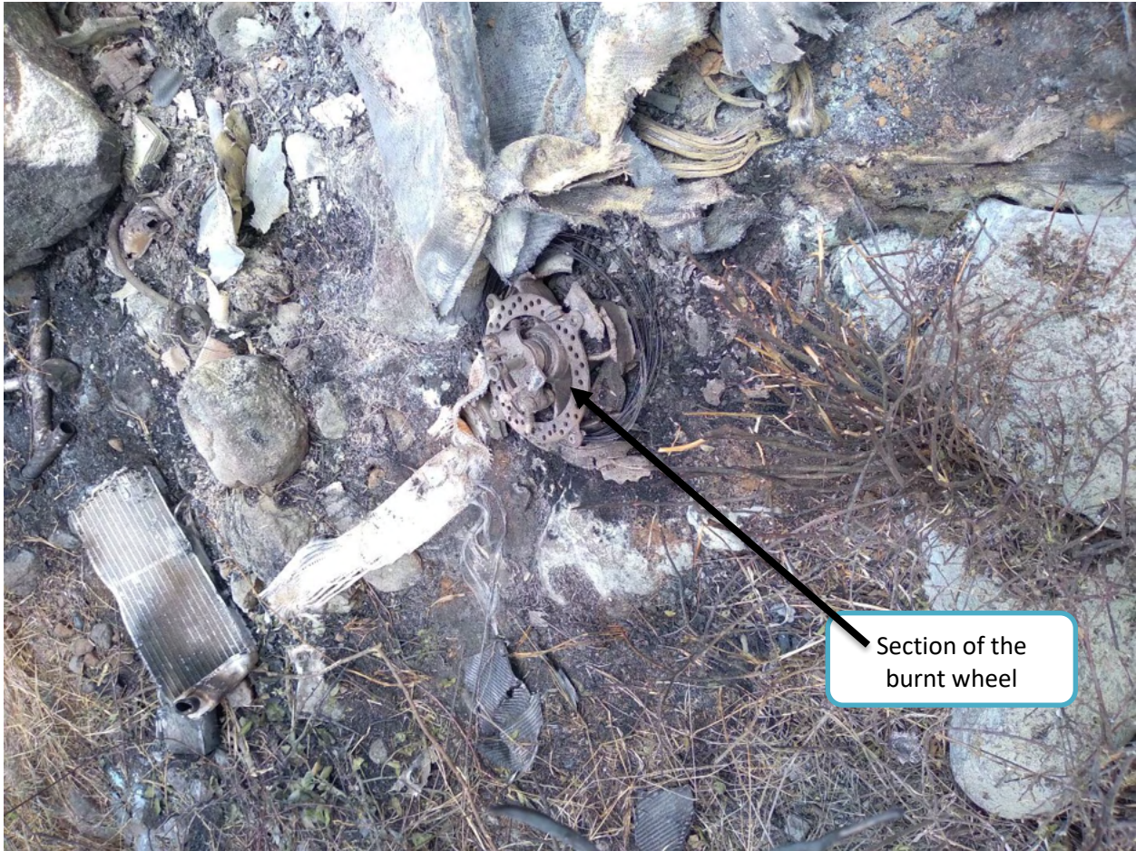
Figure 7: Photograph showing the wreckage of the burnt Gyroplane wheel assembly.
