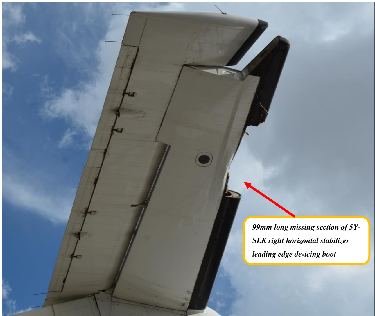
FIGURES No. 5 and 6 – Photos of the missing section of right horizontal stabilizer leading edge de-icing boot
