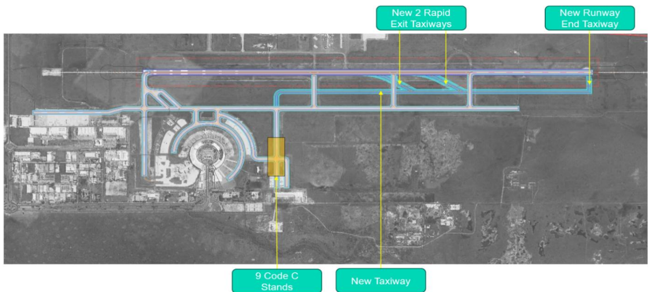
Figure 3: Improvement Works – Airfield
