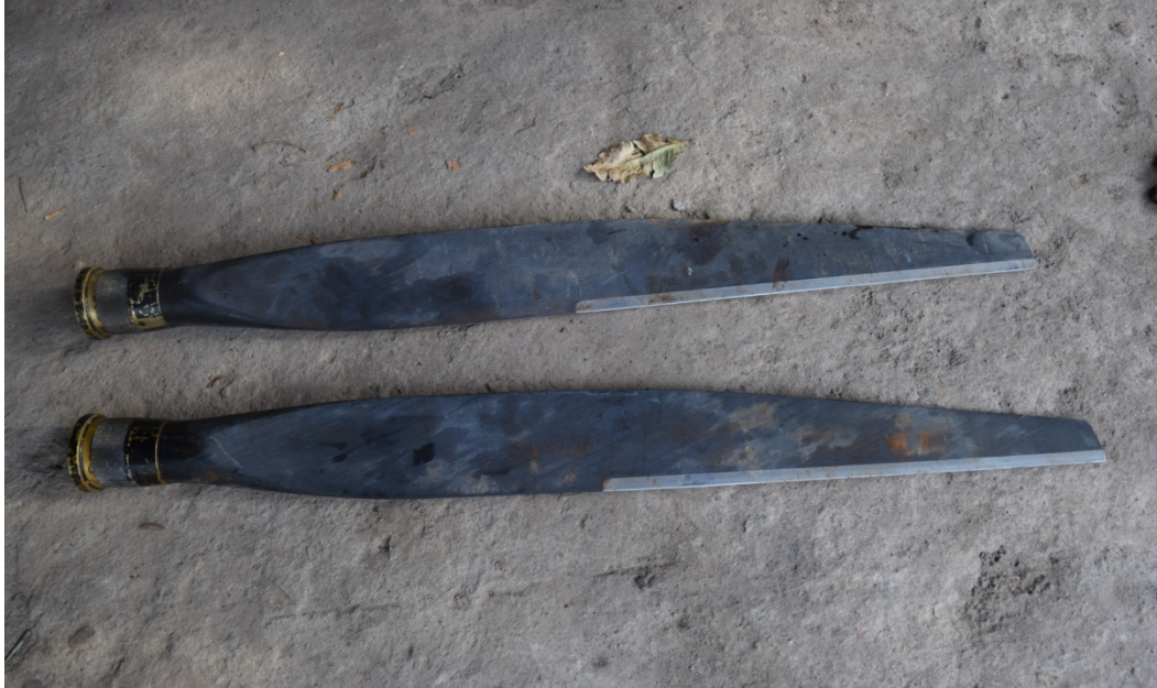
Fig 2: Propeller Blades showing normal condition
