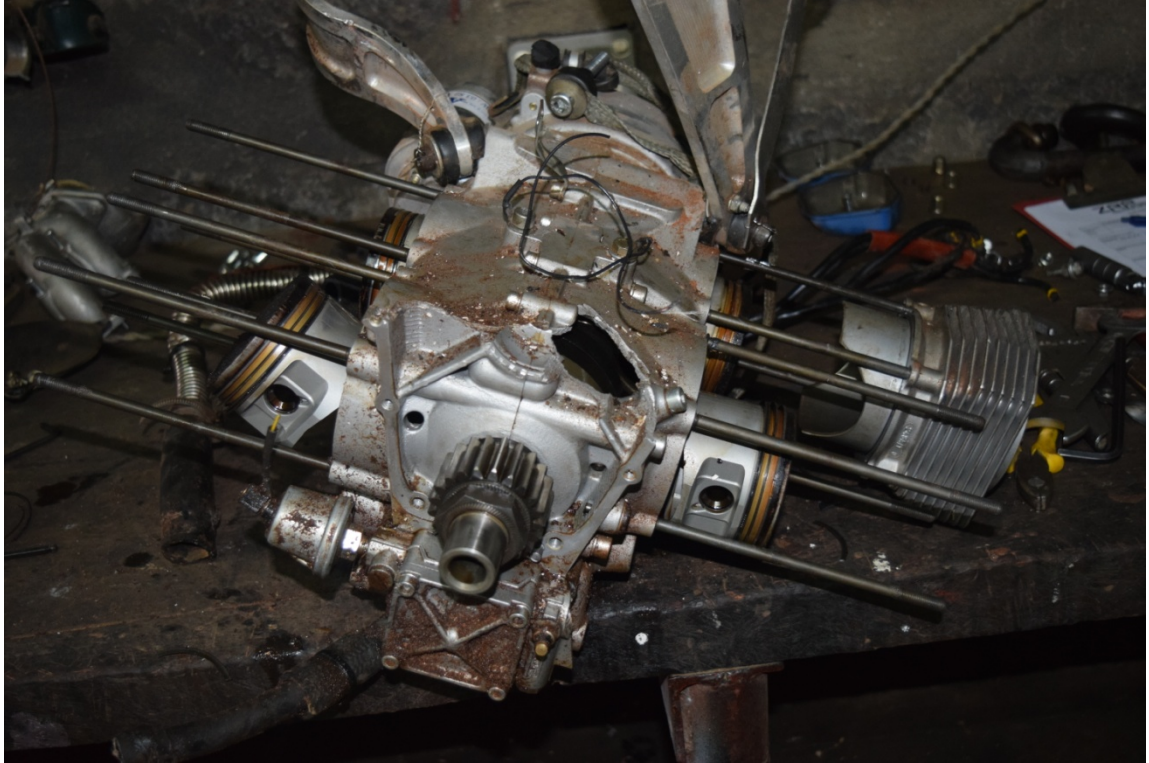
Fig 6: Surface of the Engine block showing a large hole
