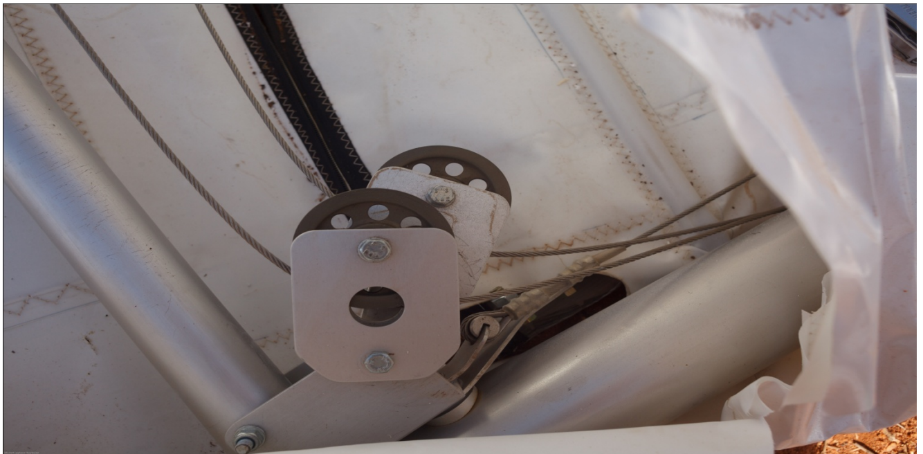
Fig. 4: Right Aileron Linkages in Place
